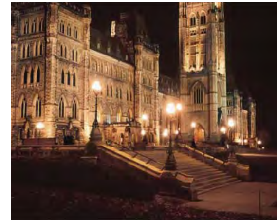
Parliament Hill Stairs: Very low quantities of light from historical pedestrian fixtures invite visitors up the stairs. Soft vertical light on the buildings gives a feeling of comfort and good visibility. Maximum illumination is 10 lux with minimums under 1 lux.
