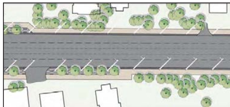
Atypical Detail Plan: North of Steeles Station - Asymmetrical boulevards, sidewalks flank road on both sides.
