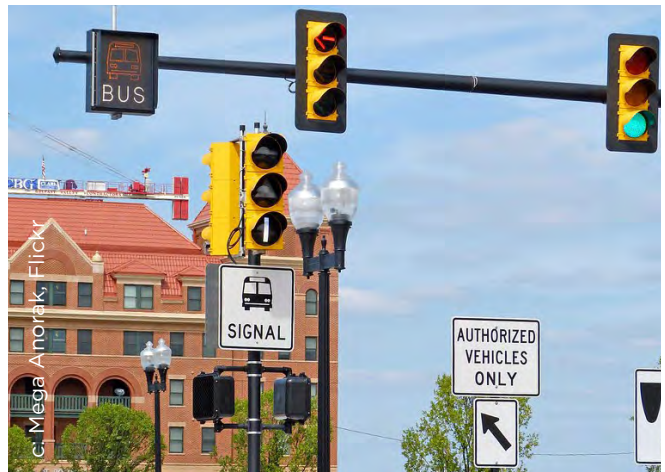
Figure 4.50. Traffic signals and signage for different users.
