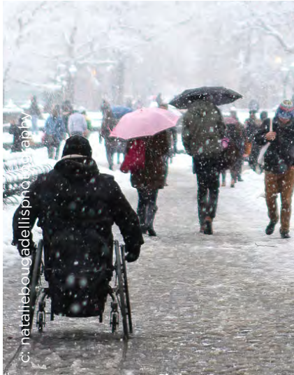
Figure 2.36. Designing streets that consider four season use means ensuring clear and accessible facilities for all users, and providing enough space for snow storage while maintaining suitable pedestrian clearway.
