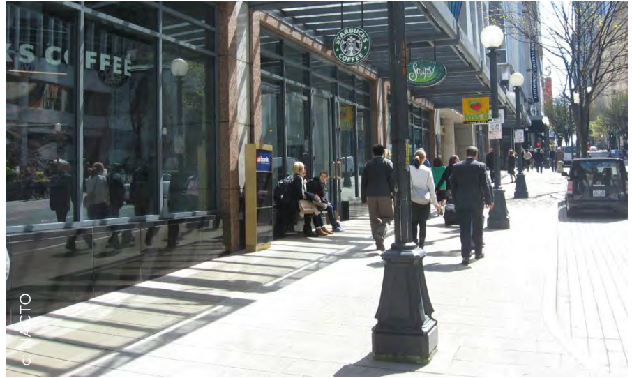
Figure 4.5. Boulevard in mixed-use areas to have wider pedestrian clearway to accommodate higher pedestrian volumes.
