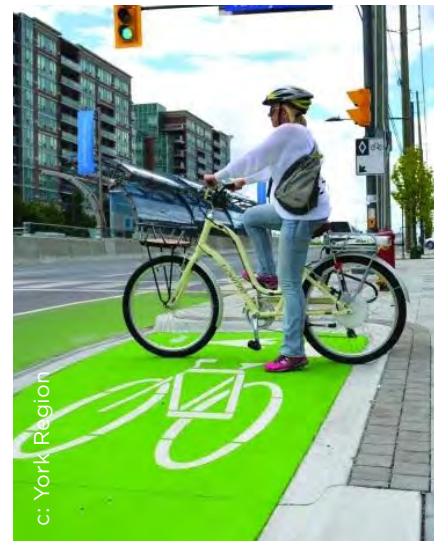
Figure 2.28. Left turn bike box is an example of preventing conflicts arising from cyclists queuing in a cycle lane or a crosswalk.
