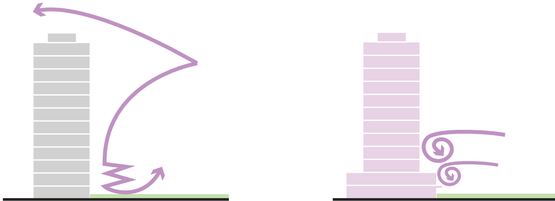
Figure 191. Left: Accelerated wind speeds create undesirable windward corners. Right: Tower that is setback from the base reduces undesirable downward wind flow.
